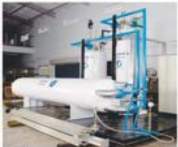
COPS-COVERGAS PURIFICATION SYSTEM AT IGCAR
